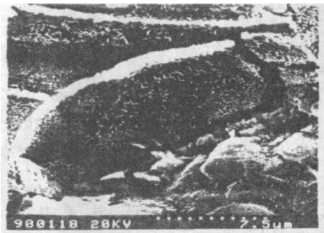
Fig.8 SEM micrograph of interfacial zone for reactive aggregate-bearing mortar at 2% CaCl 2
