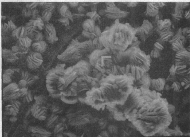
Fig. 4c - AAR rosettes formed on a reacted basalt particle in the mortar bar
