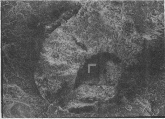
Fig. 4a - AAR product filling a void in the mortar bar subjected to the AMBT
